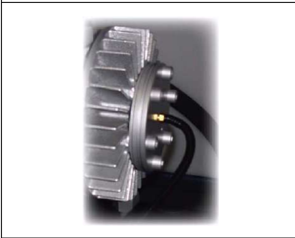
Figure 5-13 High Temperature Switch
